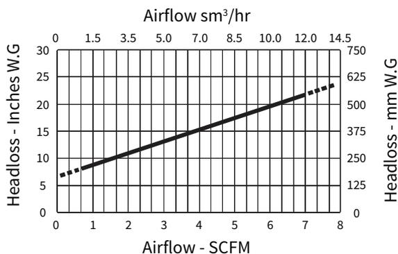
\*Installations under 2 SCFM/3.5m³/hr should consider an orifice plug to ensure uniform air distribution
